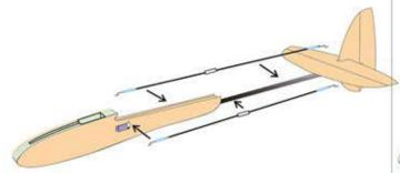
Connect the control rods to the servos and control horns.
